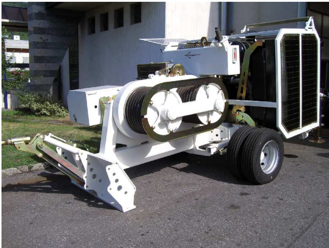
Mod. 107/18/R HYDRAULIC PULLER FOR CONTINUOUS CONDUCTORS STRINGING OPERATION
